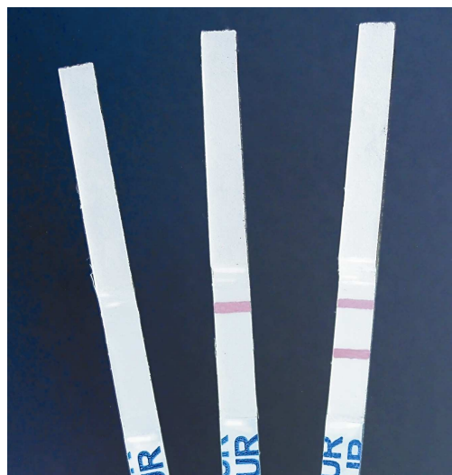
Example of an unreacted, negative (1-line) and positive (2-lines) test strip
